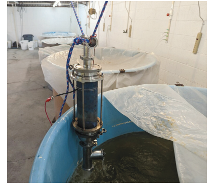
The Aquaculture Pathology Lab is testing a new design of photocatalyst to disinfect water in commercial applications.
